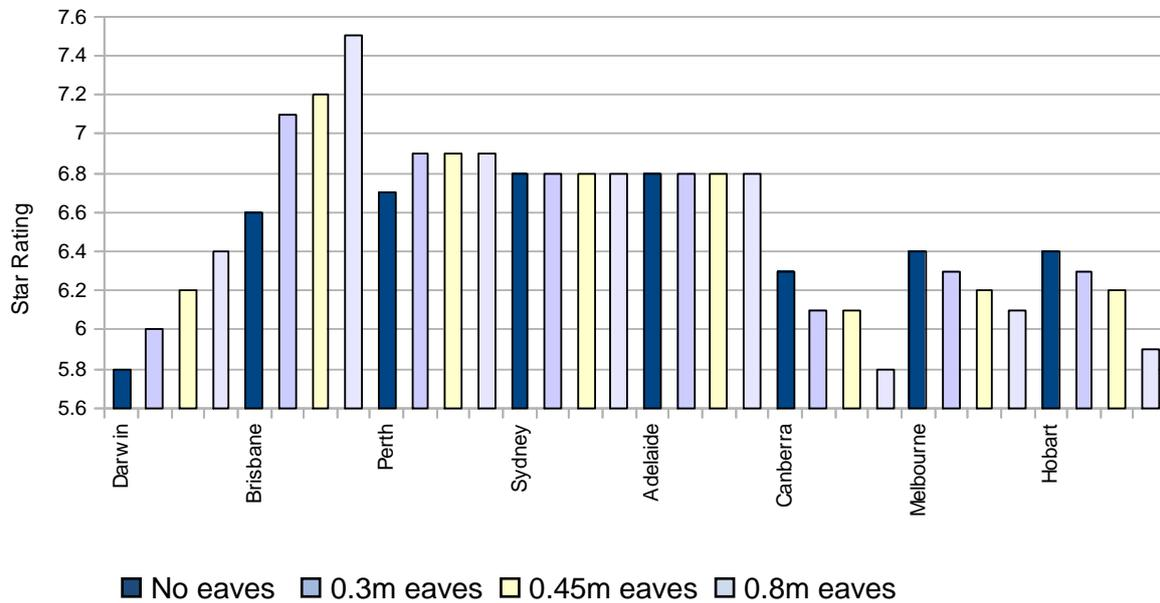
**Figure 23: The effect of eave width on star rating for a single storey detached house ( Dwelling 2 ) in each capital city.**
