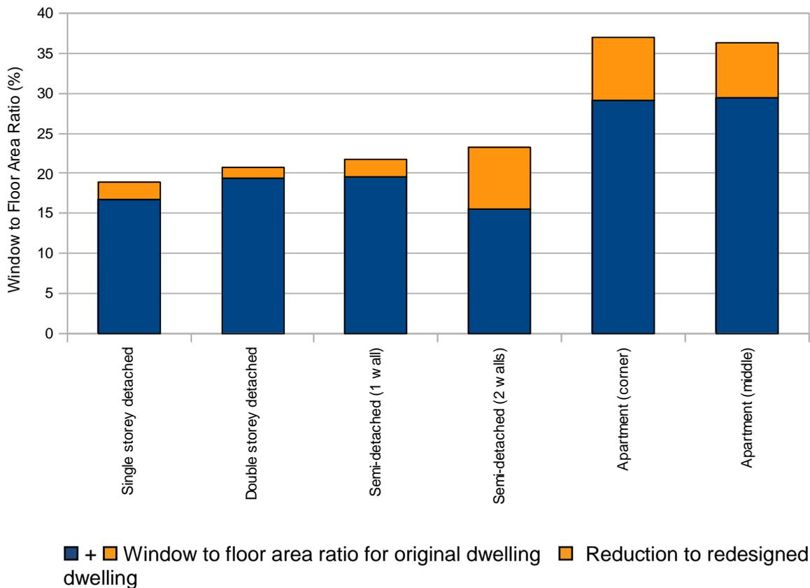
**Figure 13: Window to floor area ratio by dwelling type for the original design and reduction due to redesign.**
