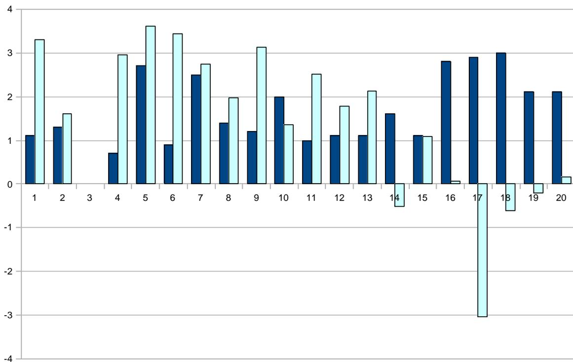
**Figure 30: Star rating change and cost saving (%) in Brisbane for each dwelling as a result of redesign changes.**
