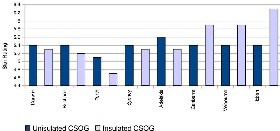
**Figure 21: The effect of uninsulated and insulated CSOG on star rating for a double storey detached house (Dwelling 8) in each capital city, where the main living area has vinyl floor covering.**
