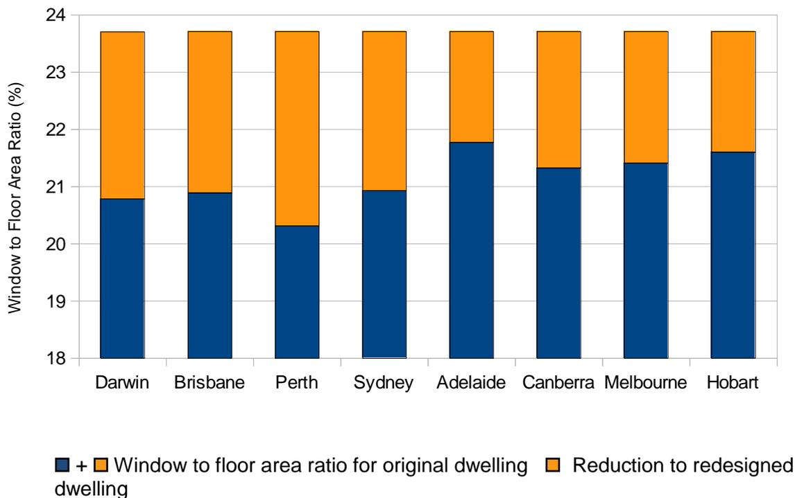
**Figure 14: Window to floor area ratio by capital city for the original design and reduction due to redesign.**
