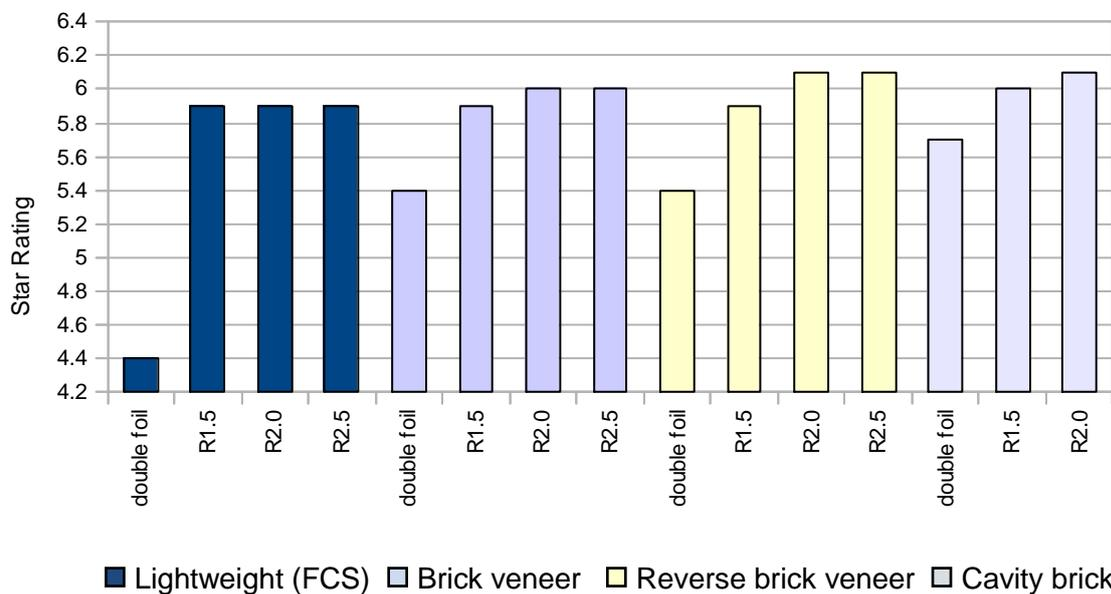
**Figure 25: Comparison of the effect of wall construction and insulation on star rating for a single storey detached house (Dwelling 2) in Darwin.**
