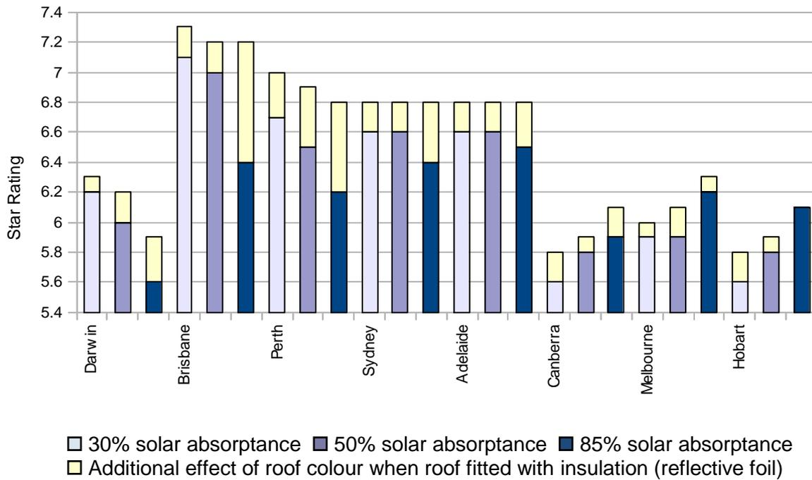
**Figure 17: The comparative effect of roof colour when the roof has no form of insulation and with reflective foil to the roof on star rating for a single storey detached house (Dwelling 2) in each capital city.**
