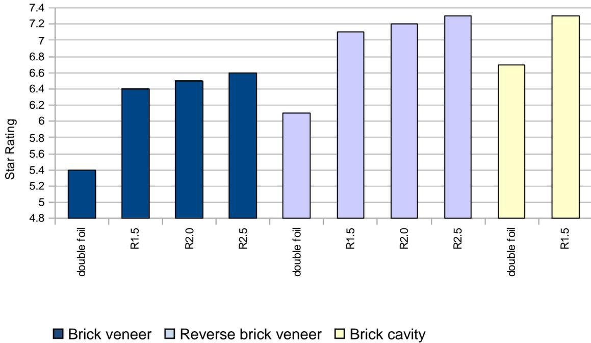
**Figure 26: Comparison of the effect of wall construction and insulation on star rating for a single storey detached house (Dwelling 4) in Perth.**
