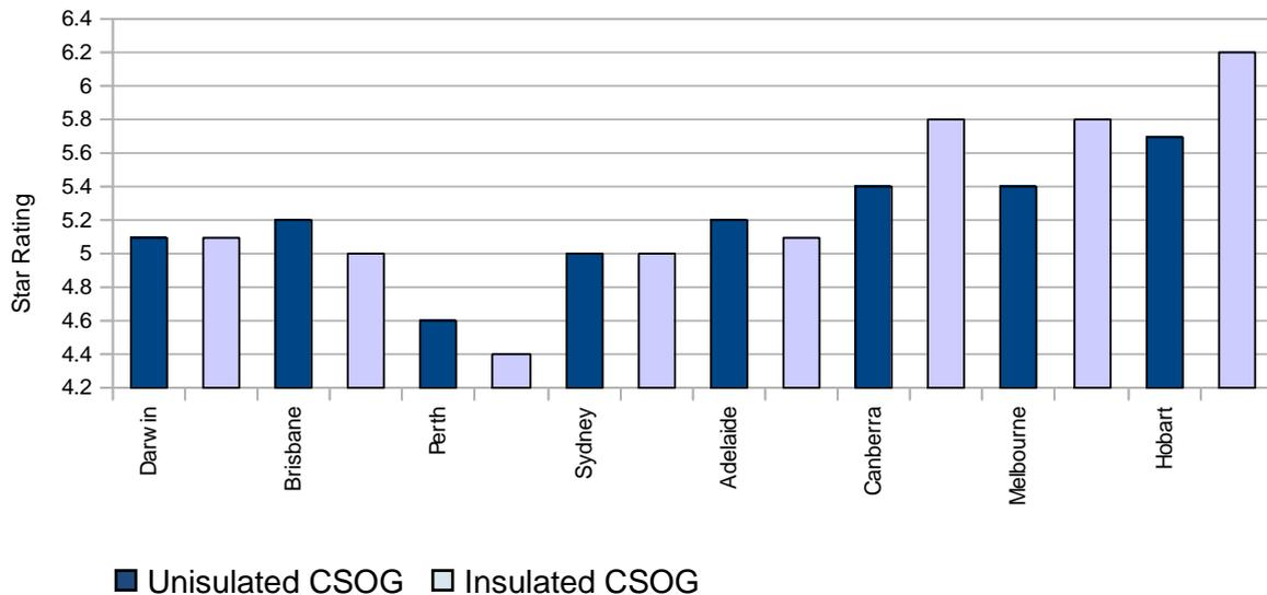
**Figure 22: The effect of uninsulated and insulated CSOG on star rating for a double storey detached house (Dwelling 8) in each capital city, where the main living area has carpet floor covering.**
