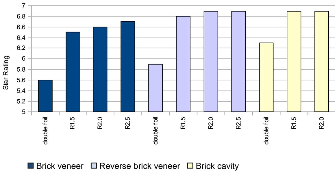
**Figure 27: Comparison of the effect of wall construction and insulation on star rating for a single storey detached house (Dwelling 4) in Melbourne.**
