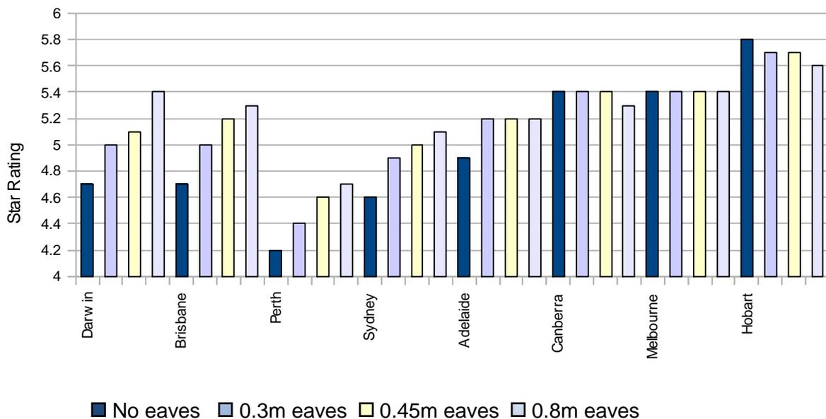
**Figure 24: The effect of eave width on star rating for a double storey detached house ( Dwelling 8 ) in each capital city.**
