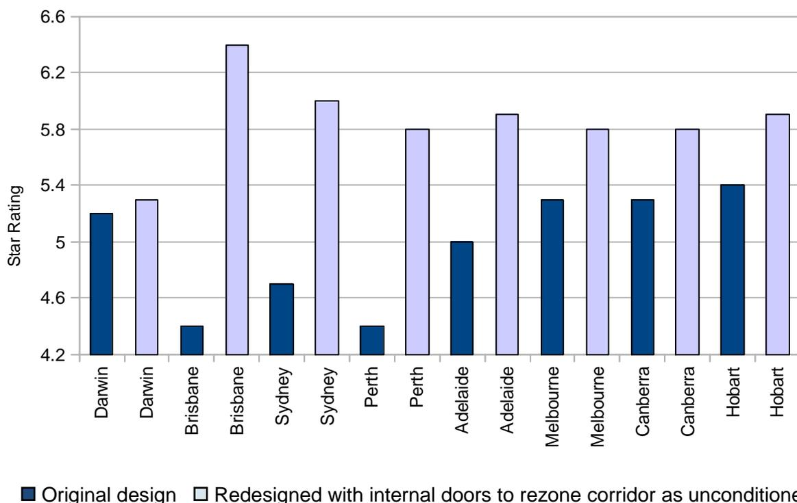
**Figure 16: Star rating in all capital cities for a double storey detached house (Dwelling 12) illustrating the impact of using internal doors to rezone 56m<sup>2</sup> of corridor as unconditioned space.**
