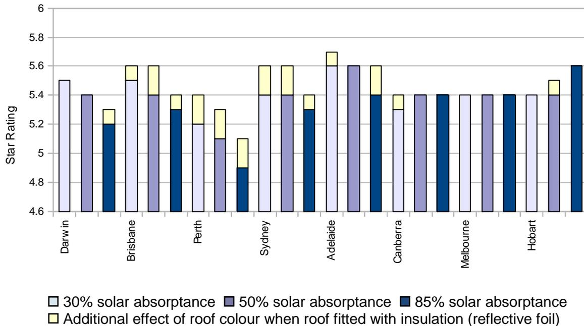
**Figure 18: The comparative effect of roof colour, when the roof has no form of insulation and with reflective foil to the roof, on star rating for a double storey detached house (Dwelling 8) in each capital city.**
