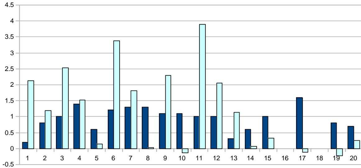
**Figure 35: Star rating change and cost saving (%) in Melbourne for each dwelling as a result of redesign changes.**
