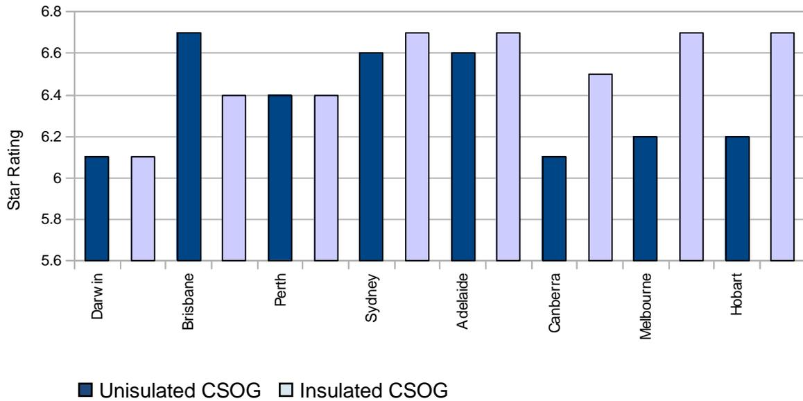
**Figure 20: The effect of uninsulated and insulated CSOG on star rating for a single storey detached house (Dwelling 2) in each capital city, where the main living area has carpet floor covering.**
