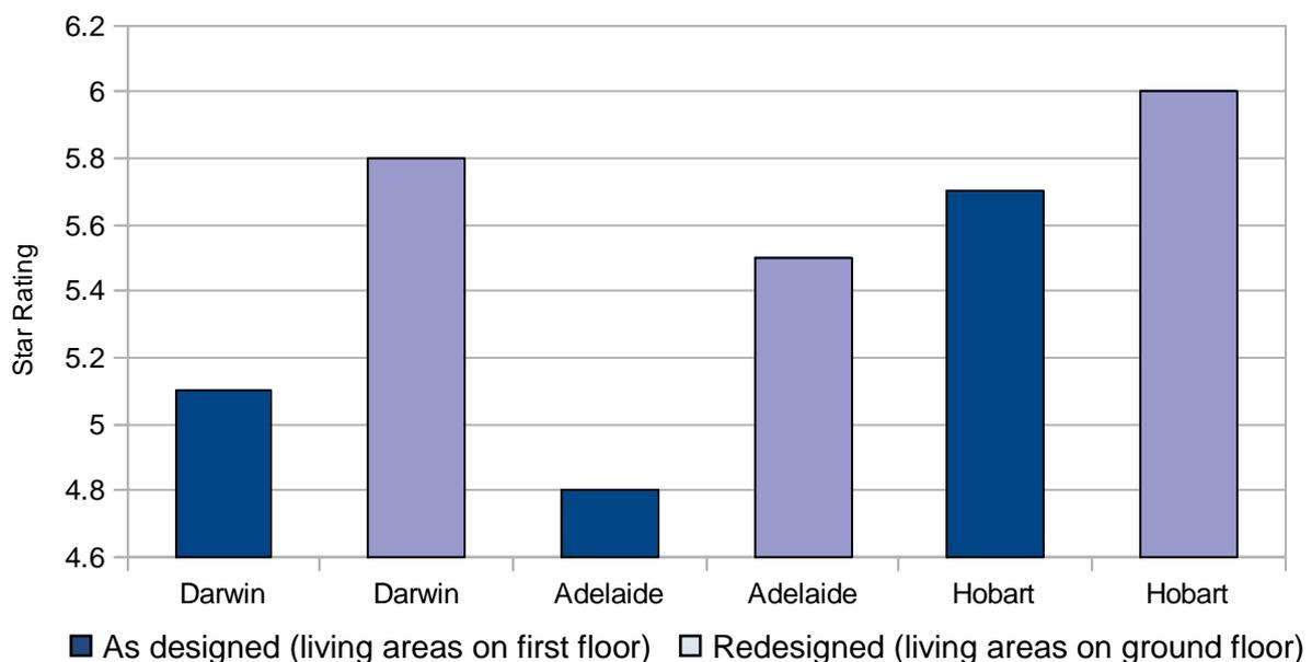
**Figure 15: Star rating change for a double storey detached house (Dwelling 10) as designed with living areas on the upper level and bedrooms on the ground level compared to as redesigned with living areas on the ground level and bedrooms on the upper level in three capital cities which represent the three climate types in this study.**
