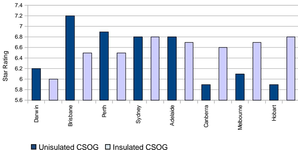
**Figure 19: The effect of uninsulated and insulated CSOG on star rating for a single storey detached house (Dwelling 2) in each capital city, where the main living area has vinyl floor covering.**
