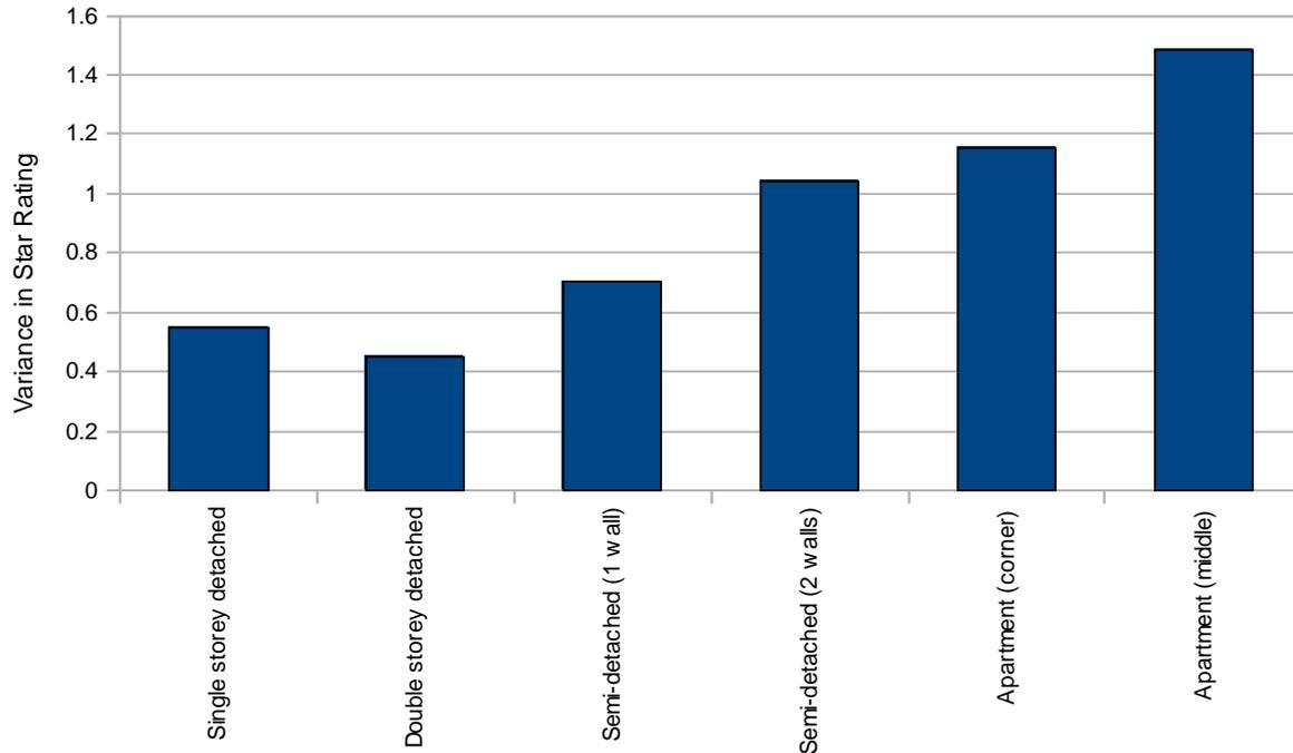
**Figure 3: Variance in star rating due to orientation for original designs averaged by dwelling type.**
