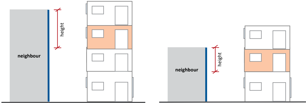
Figure 9-14 Elevations of vertical shading height for Class 2 dwellings*
