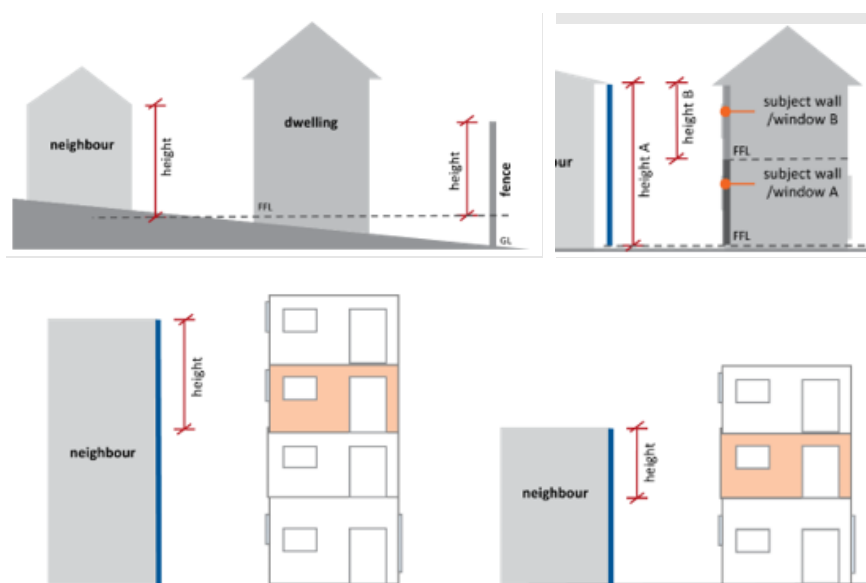
Figure 10.4 - Vertical shading – height
