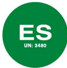
Figure 18.2 - Switchboard signage indicating battery chemistry
