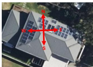
Figure 17.4 - Estimating array orientation
