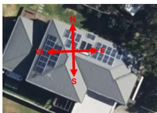
Figure 17.4 - Estimating array orientation
