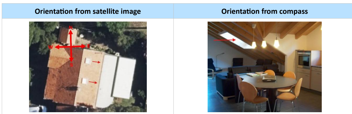
Figure 8.1 - Determining orientation of skylights/roof windows
