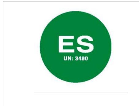
Figure 7 - Switchboard signage indicating battery chemistry
