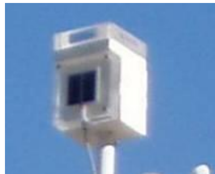
Figure 3.42 – SolData 80SPC pyranometers measuring global and north vertical solar radiation
