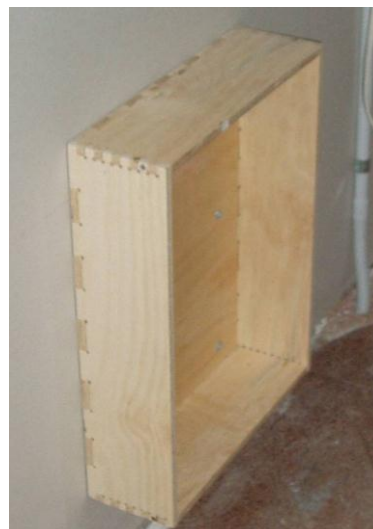
Figure 2.49 - The heater mounting box fixed to test cell internal wall
