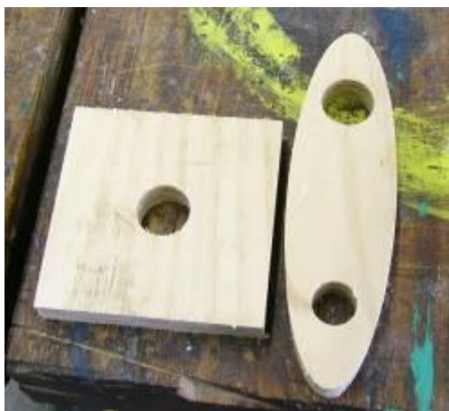
Figure 3.27 – CNC router-cut bottom or top plate and ovoid environmental sensor support
