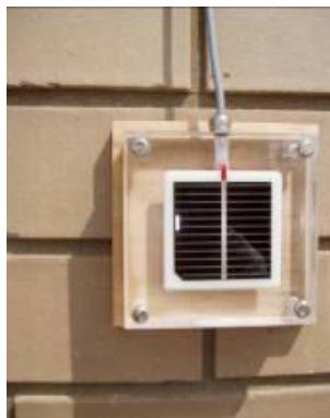
Figure 3.41 - The SolData 80SPC pyranometer affixed to brick veneer wall
