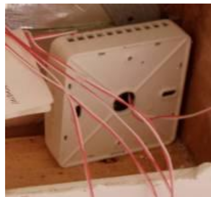
Figure 3.19 – HMW40U relative humidity transmitter installed within a test cell wall cavity
