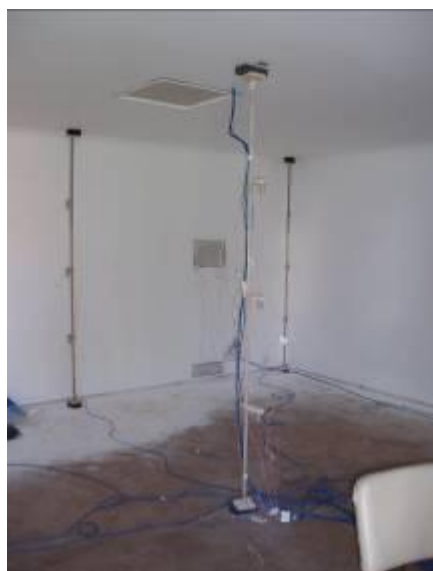
Figure 3.29 – Adjustable pole in centre of test cell room with AD592CN temperature sensors at 600mm, 1200mm and 1800mm
