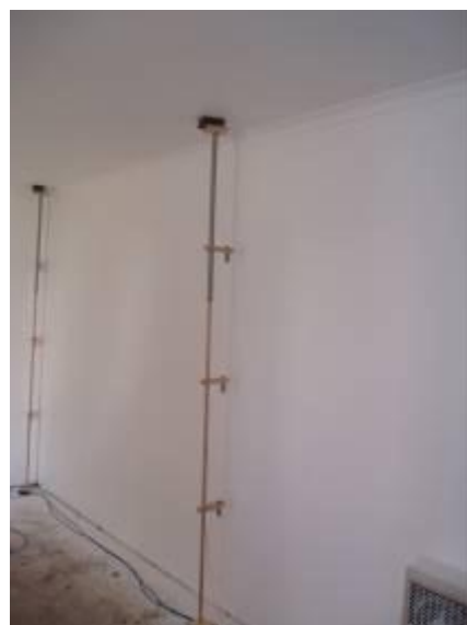
Figure 3.30 – Adjustable pole along western wall of test cell room with AD592CN temperature sensors at 600mm, 1200mm and 1800mm
