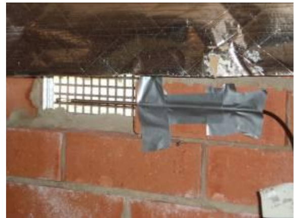
Figure 3.24 - Airflow measurement (close view) through subfloor air vent of the test cell
