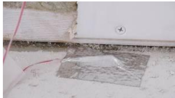
Figure 3.10 – Surface temperature measurement: AD592CN probe affixed to floor and covered with reflective tape
