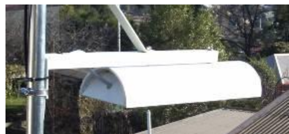
Figure 3.39 – The radiation and rain shield of the Vaisala HUMICAP HMP45A/D combined temperature and humidity probe viewed from above
