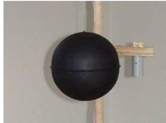
Figure 3.17 – After painting, completed copper globe sensor in place
