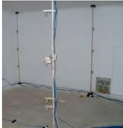
Figure 3.15 – Adjustable poles within test cell showing air temperature measurement at 600mm, 1200mm, 1800mm air temperature and relative humidity at 1200mm
