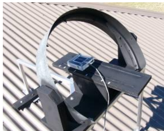
Figure 3.44 – SolData 80SPC pyranometer as part of shadow ring device for measuring diffuse solar radiation
