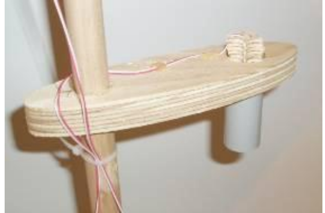
Figure 3.14 – AD592CN temperature probe installed within 25mm PVC tube
