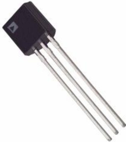
Figure 3.5 –AD592CN as supplied
