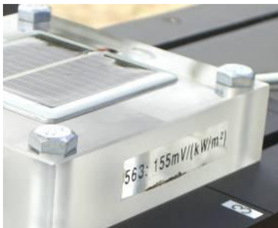
Figure 3.43 – SolData 80SPC pyranometer serial number 563 with a span value of 155mV = 1.0KW/m 2
