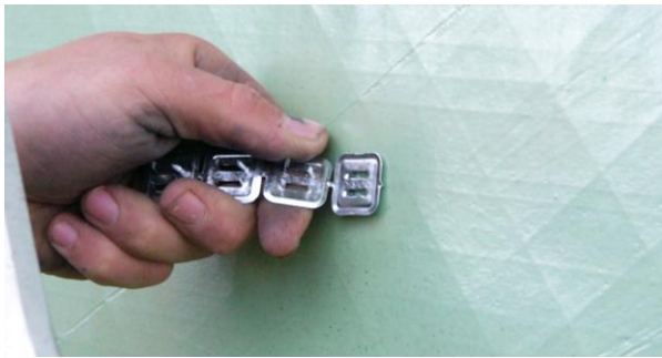
Figure 2.25 - Steel staples used to affix building wrap and roof sarking
