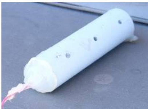
Figure 3.11 – The final type of in-ground temperature probe within a silicone-filled tube
