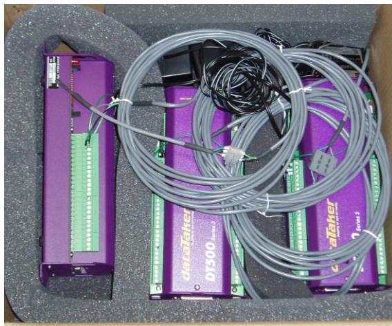
Figure 3.47 – New DT500 data loggers and channel expansion modules
