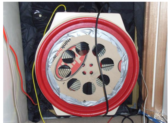
Figure 3.38 - View of the pressurisation fan of the blower door equipment
