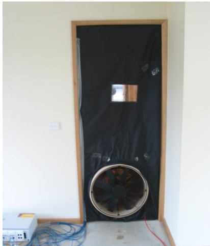
Figure 3.37 - Interior view of the blower door equipment installed in the case study house
