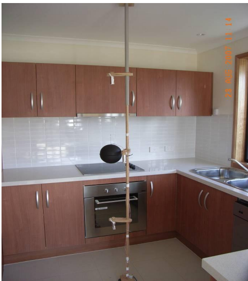
Figure 3.12 - Timber pole with temperature sensors located at different height levels
