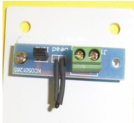
Figure 3.10 - AD 592 CN temperature sensors attached to wall plate at the wall
