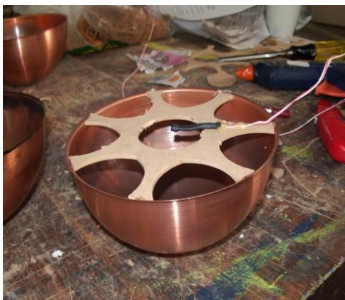
Figure 3.30 - Inserting the air temperature sensor into the globe half sphere
