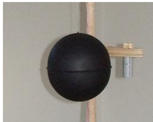
Figure 3.31 - Globe thermometer installed and measuring environmental temperature
