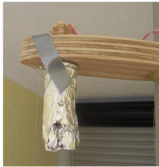
Figure 3.13 - Temperature sensor fixed inside a plastic pipe, covered by reflective foil
