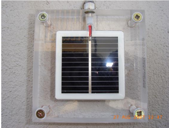
Figure 3.33 - SolData 80SPC pyranometer fixed to an external wall
